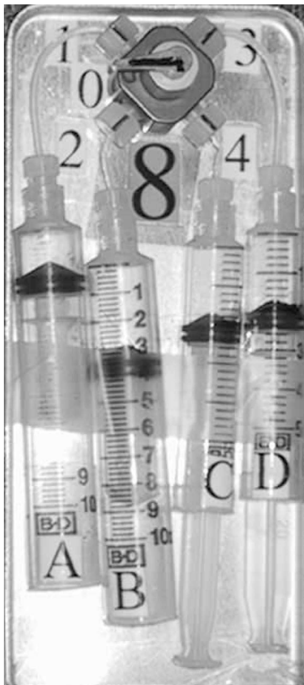
Figure 1 BPM photograph. Sterile medium (6 ml) was loaded into syringe A, inoculum in seed medium (2 ml) in B, and a fixative (ethanol, 1.5 ml each) in C and D.
